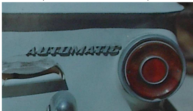
Below: close-up of 1968 Automatic with upper-case script and late-model tail light base (but with incorrect earlier lens).
