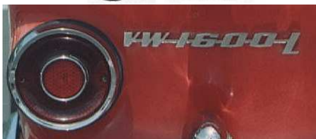
Above: Correct for 1967, new VW1600L script with earlier style tail light & solid red early style lens.
