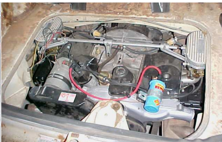
Doug Gray.....Elizabeth, Colorado USA.....1962 343 (0 042 990) 1641cc & baby Dell's, 12 volt, converted to 4 lug with Type 4 rotors/calipers, 1968 Type I tranny with T3 axles
