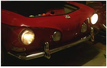
Above comparison: the left bulb is a 6V sealed beam, while the right one is the new 6V halogen convex producing twice the light! Makes a huge difference at night!
