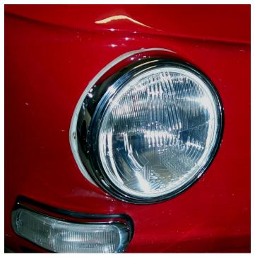
The reflectors are made by Valeo, the 6V bulbs by Narva, and they mount into your existing T34 headlight assembly. Original sealed-beam 6V bulbs burn at 500 lumens and these new 6V halogen bulbs burn at 1000 lumens low-beam & 1650 lumens high-beam!
