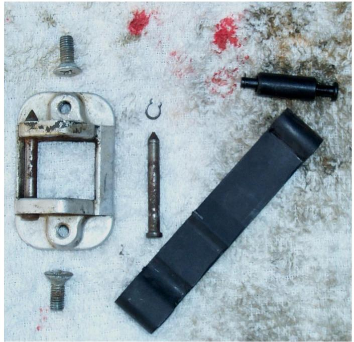
Next I found it necessary to grind-down the edges of the rollers to fit the T34 retaining plate. I also found that only one roller was needed, not both. Each check strap is marked with an L or R to show which side goes up. Install the check strap (fat end towards the back of the car), pins, roller, & circlips.
