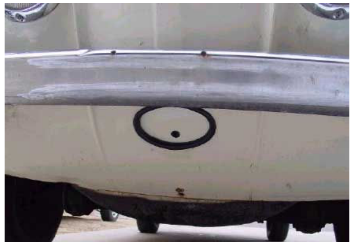
Late style: metal cover plate & seal with second L-tube
