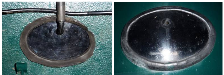
Late style: metal cover plate & seal with second L-tube
