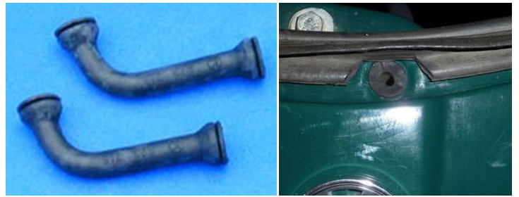
Repro front drain L-shaped tubes & tube installed in drain hole
