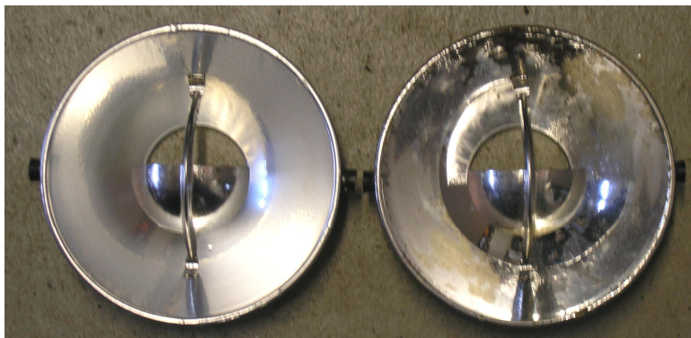
Restored fog light reflector (left) to an original (right).
