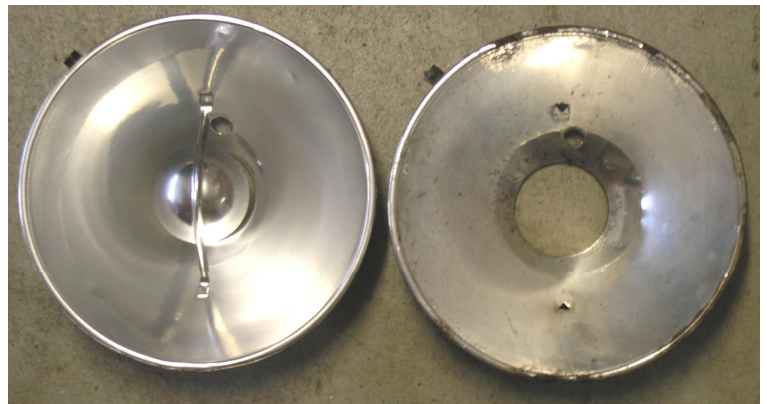
Restored headlight reflector (left) to an original (right).
