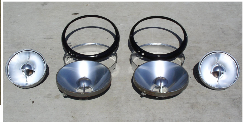
Restored headlight reflector (left) to an original (right).
