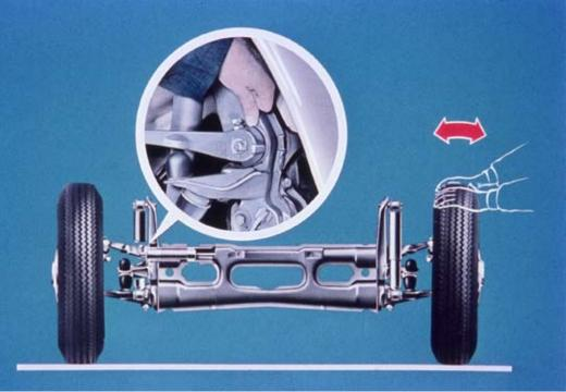
18/43 – The upper torsion arms of the front axle are connected by the stabilizer and must not have any exial play. The play is checked as follows: We bounce the vehicle at the front and rear so that the wheels are no longer in a loaded condition.
