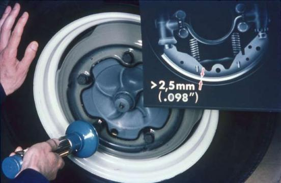
18/16 – Regular checking of the brake linings is an important contribution to the road safety of a vehicle. As in the case of Type 1, we check the lining thickness by shining a light through the inspection hole in the brake drums. The wear limit is .10" also.
