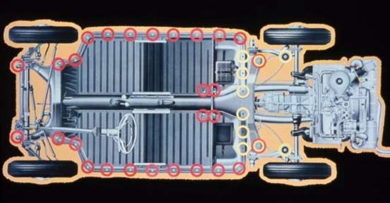
18/19 – This picture shows all the connection points between frame, subframe and body which have to be checked for tightness at the 300 mile maintenance service. If the rubber weatherstrip between frame and body is to remain supple and not be squashed by being over-tightened, the body bolts must be tightened with a torque wrench only.
