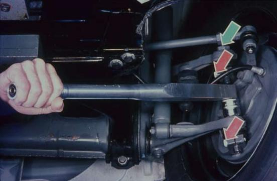
18/14 – The nuts and bolts of the front and rear axles are only tightened during the maintenance service at 300 miles.
