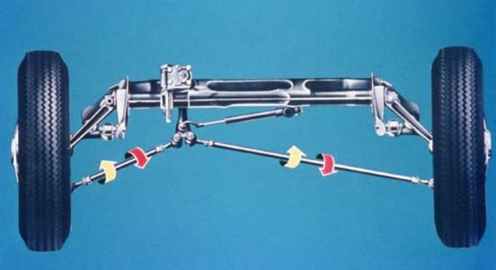
18/48 - The toe-in is adjusted by turning the tie rod tubes. Both tie rods must be lengthened or shortened by the same amount so that the center position of the steering will not be effected. By turning the tie rods in driving direction - yellow arrow - we increase the toe-in, by turning them in the opposite direction - red arrow - we reduce the toe-in. By using an optical wheel alignment gauge exact camber and toe-in settings can be achieved.
