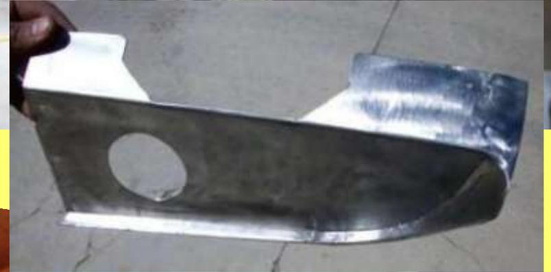
Normally if I was to media blast to remove old paint I would prefer soda blasting as it's best to keep from warping the large flat area. However with this much rust present, I opted for Silicon Carbide as it's harder but it cuts fast so it doesn't heat up the metal as much. It gets to the surface rust much better and is also a little less expensive since it can be recycled. Immediately after the car was blasted it was coated with an epoxy primer.
