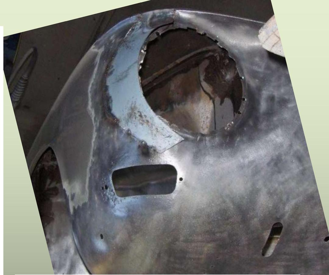
The chassis and some rear end parts were sanded-down as were the bottom and the undersides of the fenders of the T34 body. Franck didn't want to sand the whole body because he was afraid of metal distortion. The sanding exposed the rust damage which was more body work than Franck expected. The worst rust was in the headlight buckets, spare tire well, and at the bottom of the fenders, but the chassis was in good condition with only minor rust on the sides.
