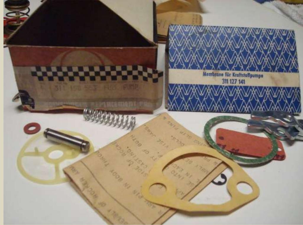
Above: the complete kit #311 198 553 and the diaphragm is #311 127 141 (blue box). The complete kit includes base gaskets, fuel filter, spring, top screw gasket, and other parts.
