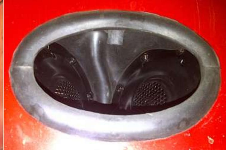
Above: with the new rubber boot fitted you can see how the long drain tube fits into the hole to drain water out of the car. Here's a low-mileage original 1964 showing how it looked when the T34 was new. And from under the front you can see the edge of the rubber boot, the dual horns, and the tip of the drain tube.
