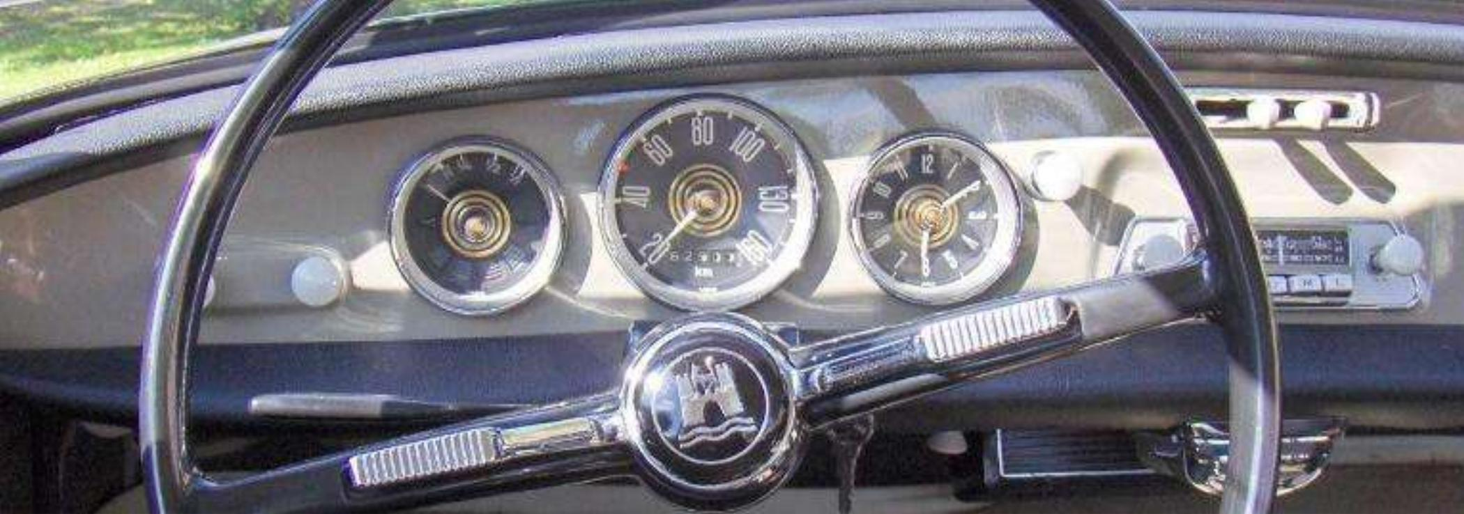
1965 Instrument Panel: The gauges in 1965 feature bronze knobs & circles, white needles, and the enlarged speedometer. The straight horn bar was continued from 1964 but would not be carried over into 1966. The pull-knobs for the lights & wiper switches were mounted into a new dash metal design. And the cigar lighter position was raised for an unknown reason, but likely to make space for the optional emergency flasher switch that could be added to the dash.
