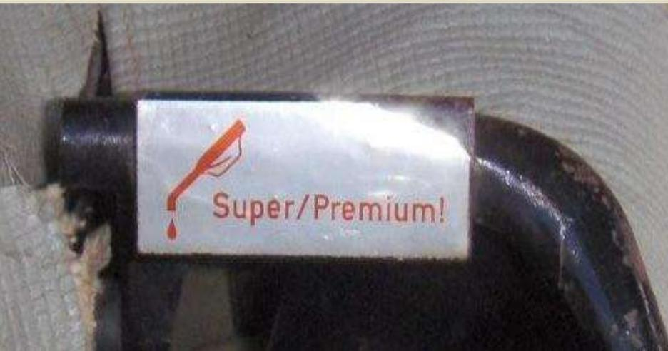
Above: the Super/Premium fuel decal & mounting plate began in mid-1964 and continued through 1965 production. It was a warning to owners to use high-octane gasoline which was required for the high-compression domed-topped pistons in the 1500 S model engines. Owners complained that the S model engines would ping and perform poorly when filled with low-octane gas. Thus this decal was fitted.
