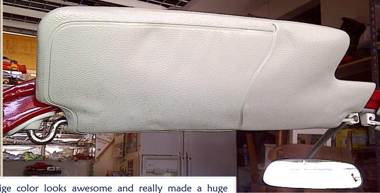
The Silver-Beige color looks awesome and really made a huge difference over the old stained visors. I lubed the chrome arms before mounting them into the visor pad holes, then tightened the set-screw to get the right amount of tension on the arm to keep the sun visor in-place while driving. The next step will be to have the surface-rusty chrome arms rechromed.
