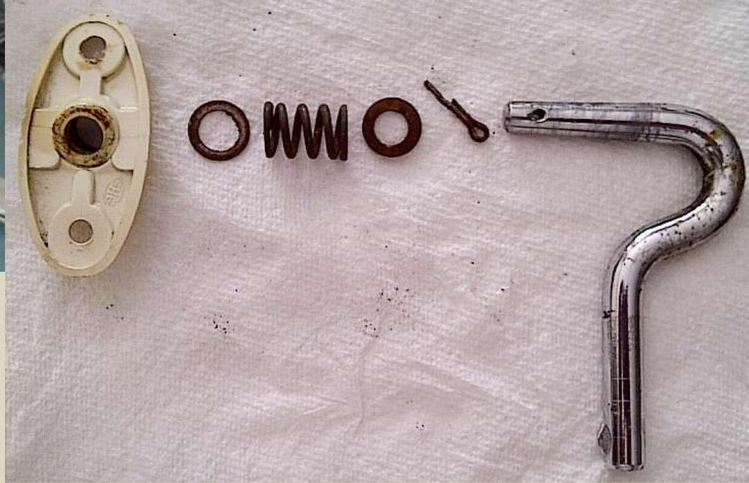
I used a degreaser on the components with a toothbrush to get them as clean as possible and then allowed them to dry completely in the sun. See the difference (bottom)? But even after cleaning it was obvious that the staining didn't look good so I made the decision to paint the parts back to Silver-Beige so they'd be correct for my 1962. The base & visors on early T34s (1962-65) is Silver-Beige and on late T34s (1966-69) is Cloud White. Wolfsburg West has spray cans of L466 Silver-Beige paint.
