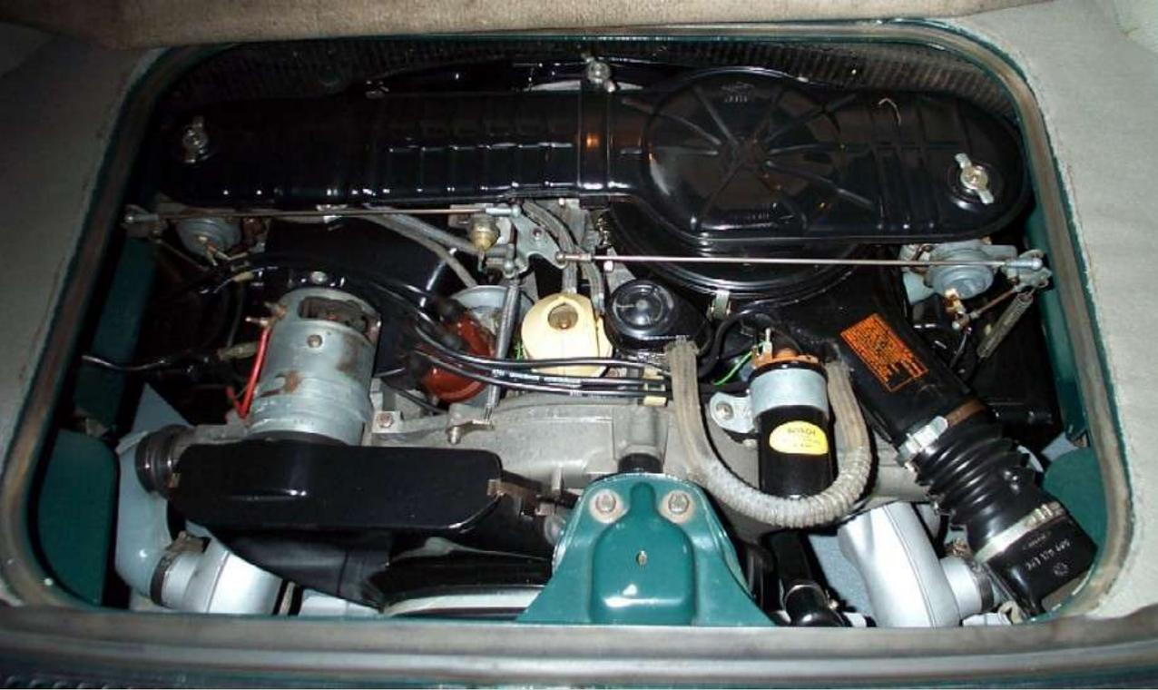
Left: The 1965 engine compartment was identical to the 1964 version with early-style fuel pump, short black 6V coil, dual carb air cleaner with rectangular decal, but the 1965 engine featured a quick-release fan belt inspection cover with clamps vs the earlier style bolts. The four-ribbed air cleaner boot was continued from the earlier design.
