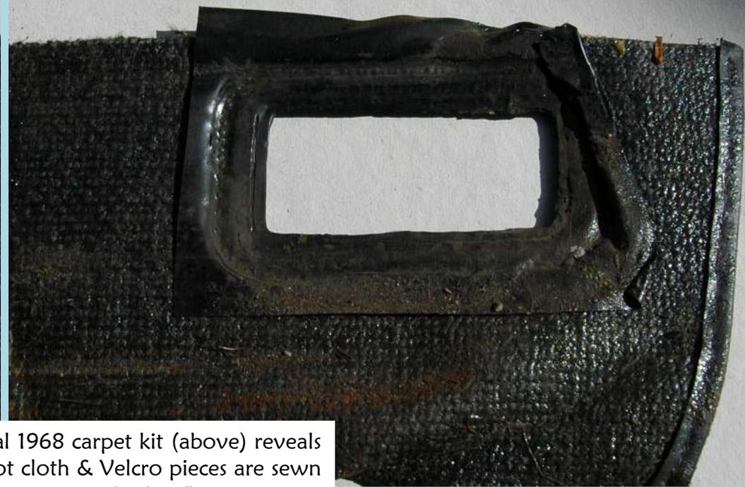
A closer inspection of an original 1968 carpet kit (above) reveals the edges are bound in vinyl, not cloth & Velcro pieces are sewn into the front heater pieces to mate with the floor mats so everything stays in-plate. He also noticed the back-side of these pieces were coated with some sort of moisture proofing that makes them much heavier than the earlier non-coated carpets.
