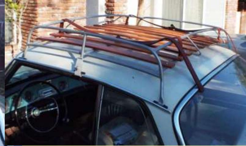
The roof racks have six feet that have black tubing to protect the gutter from scratches. There are two quick-release clamps that mount securely under the aluminum roof gutter trim. Leather straps are an optional item to give it a period-correct look. The slim profile allows air flow into electric sunroof opening also.
