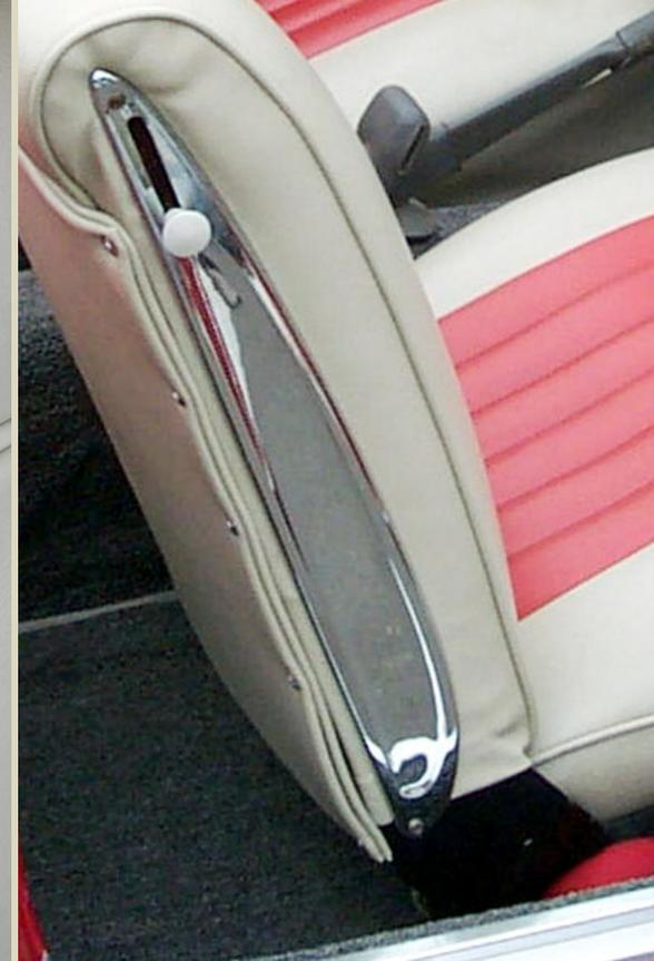
The **Mid style** (late-1962 through 1965, below) used the same ivory knob but it was relocated to the lower portion of the seat. The knob was pulled upwards to release the hook, sometimes a tough thing to do if not properly lubricated.
