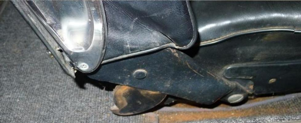
The **1966 style** (above) saw the elimination of all seat locking components and the seat was able to be folded forward at any time. Obviously this was not safe while driving and was quickly discontinued for the late-model design.
