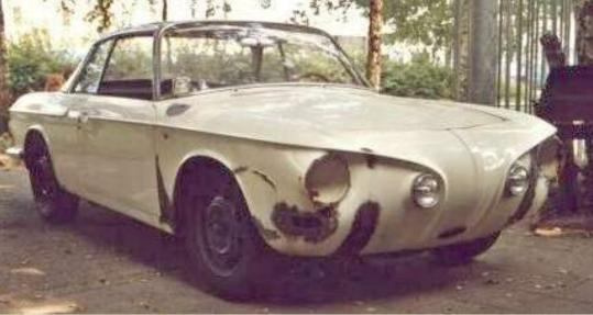
Here's the 1966 when he first found it in 2001 (above). Rusty in the front signals, bumper brackets, headlights, and wheel wells. Roel has created an eye-catching restoration since then ...
