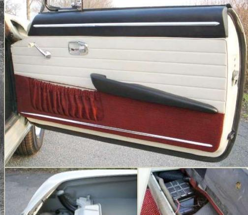
Unique to 1962 several parts are painted to match the body color: engine trapdoor metal, spare tire cover, and seat frames. The engine trapdoor cover is a solid Silver-Beige material without the Auf/Zu text or arrows. Other unique 1962 features include the solid ivory shift knob, two-piece fresh air vent trims, front seat backrest release mechanism at the top of the seats, Lemmeritz beauty trim rings that hug the outer edge of the rims, "cat's eye" side mirror, and large oil dipstick head.
