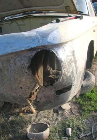
But with the windows in I decided to tackle the front end again. I pounded-out as much metal as possible but I had split a poorly welded seem under the driver's side headlight (right pic). Luckily I found a mig welder in my price range the next week. After the paint was applied the T34 was really coming along as I headed into 2011.
