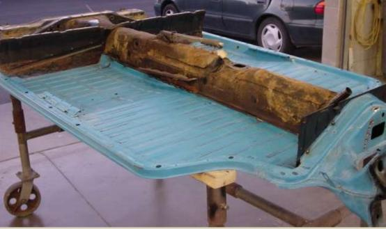
Tim separated the body from the chassis and has been working on the floorpan. He put all the factory welds back into place so it will look like it never had the pan replaced. They can't wait to drive it!
