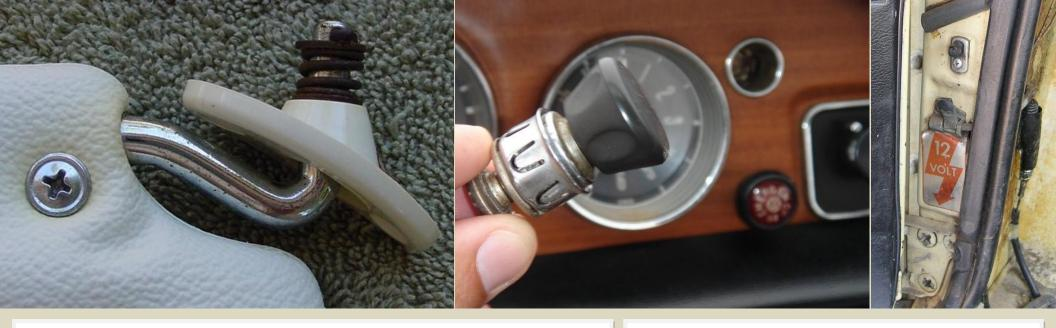
The inner door locks were moved to the top-rear of the door pads and the door pull lever became a single lever design. The aluminum trim on the door & quarter pads changed from a triangular-style to a rounded-style. The interior panels changed from the early 5-line style to a new 4-line style.
