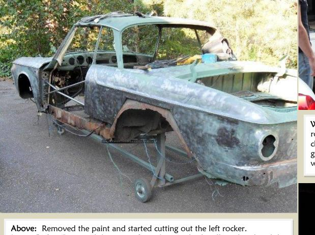
What do you plan to do next? I will finish the other side rocker panel first. Then I will put the body back onto the chassis so I can redraw the holes were the mounting screws go. I have to do it this because rust ate all the metal and it was impossible to measure from the existing holes.
