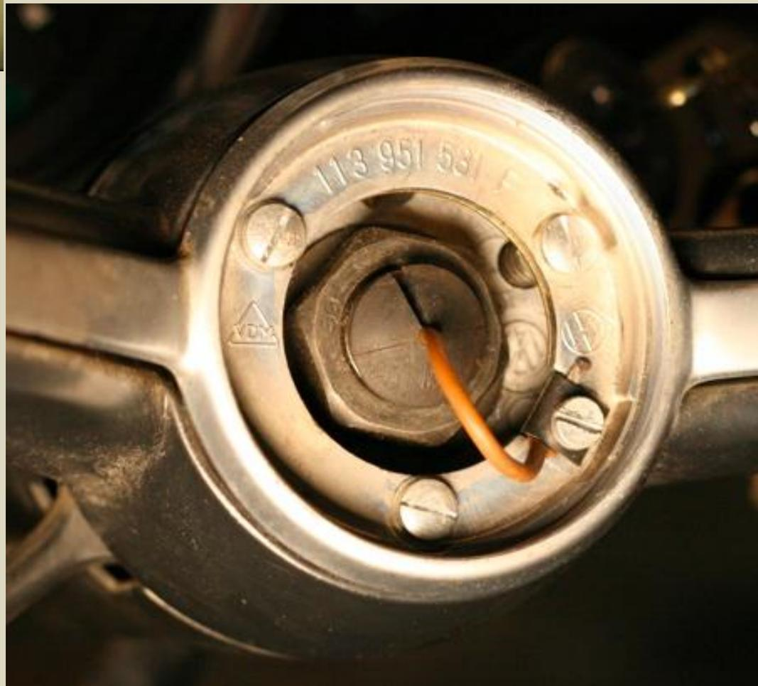
I then tracked the wire to the earthing point at the far end of the steering column just ahead of the steering box (left). Now you may be able to find this from underneath the car – but if your horn does not work then don't bother, as the easiest way is to simply undo the four bolts holding the petrol tank in place and go in from the top – where you will have much better visibility.
