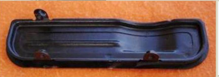
There are two different designs for the fan shroud cover plate: one secured with three bolts into the fan shroud (take more time to open & close) and one with quick-release two metal clips. appears that this inner cover seal will work well for both cover plate designs.
