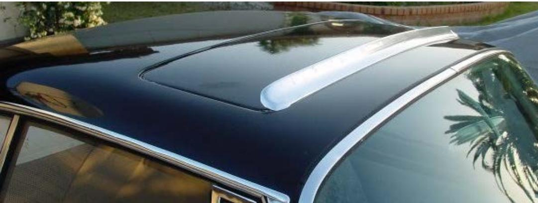
An original one (upper left) mounts to the front inner edge of the sunroof opening and is secured with screws into the roof metal. The outer edges of the deflector has a curved design. By comparison the repro deflectors has a more angled design (bottom). The repros are polished for a bright finish. Jurgen tested them on his own 1968 and fitted the felt seal over the deflector to make sure it seals properly.
