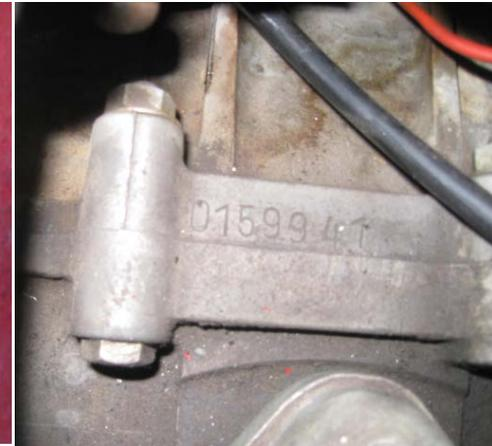
A numbers-matching T34, you can see the three VIN numbers (above). The chassis # plate is stamped under the rear seat, the body # plate is stamped into the aluminum plate inside the spare tire area, and the engine # is stamped into the engine case. Miguel's T34 has VIN # O 176 539 with original engine #O 159 941. Miguel plans to use it on an almost-daily basis from April to October except during the winter months that is usually cold and rainy in Europe.
