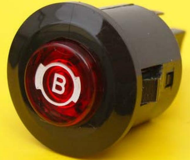
Interestingly, the metal dash panels on all late-model 1968-69 T34s were pre-stamped with the hole for the brake warning switch. But since the dash panels were covered with the wood-grained covering, the hole was not exposed until the option was fitted at the factory or at the dealer.
