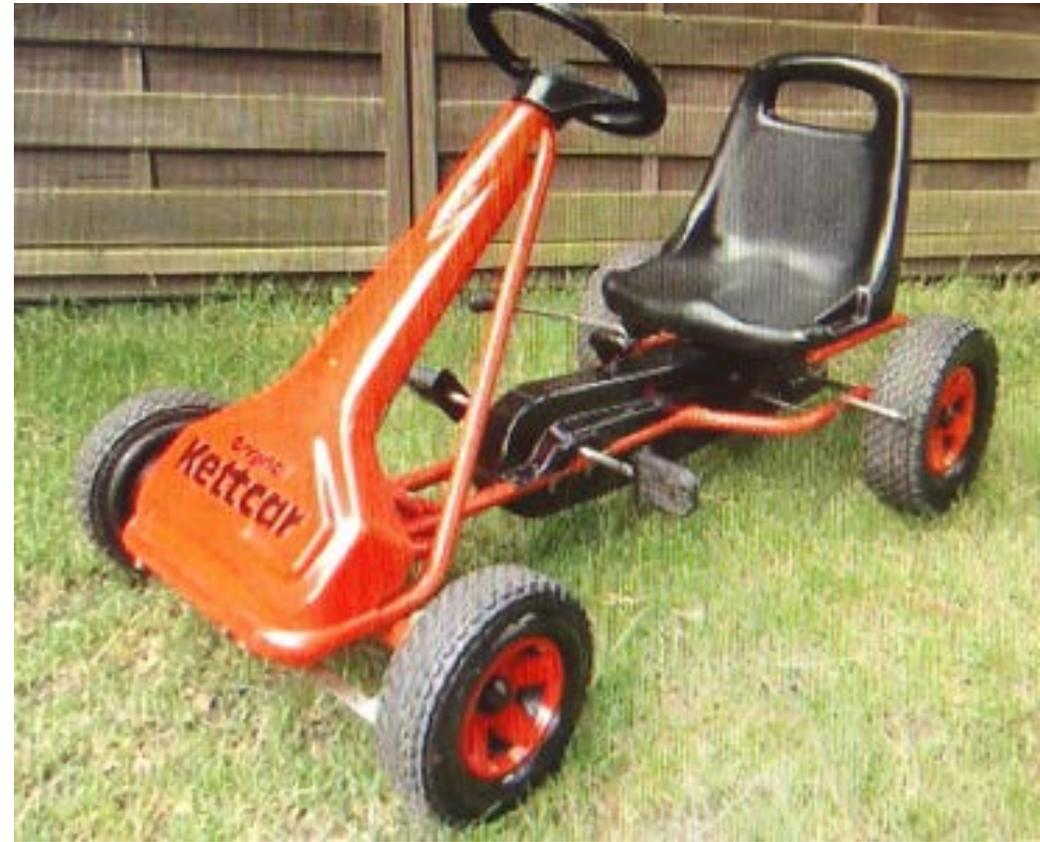
Above: The original Kettcar is a chain-driven cart with a handbrake that Matthias used as the basis for the T34 Cabriolet pedal car.
