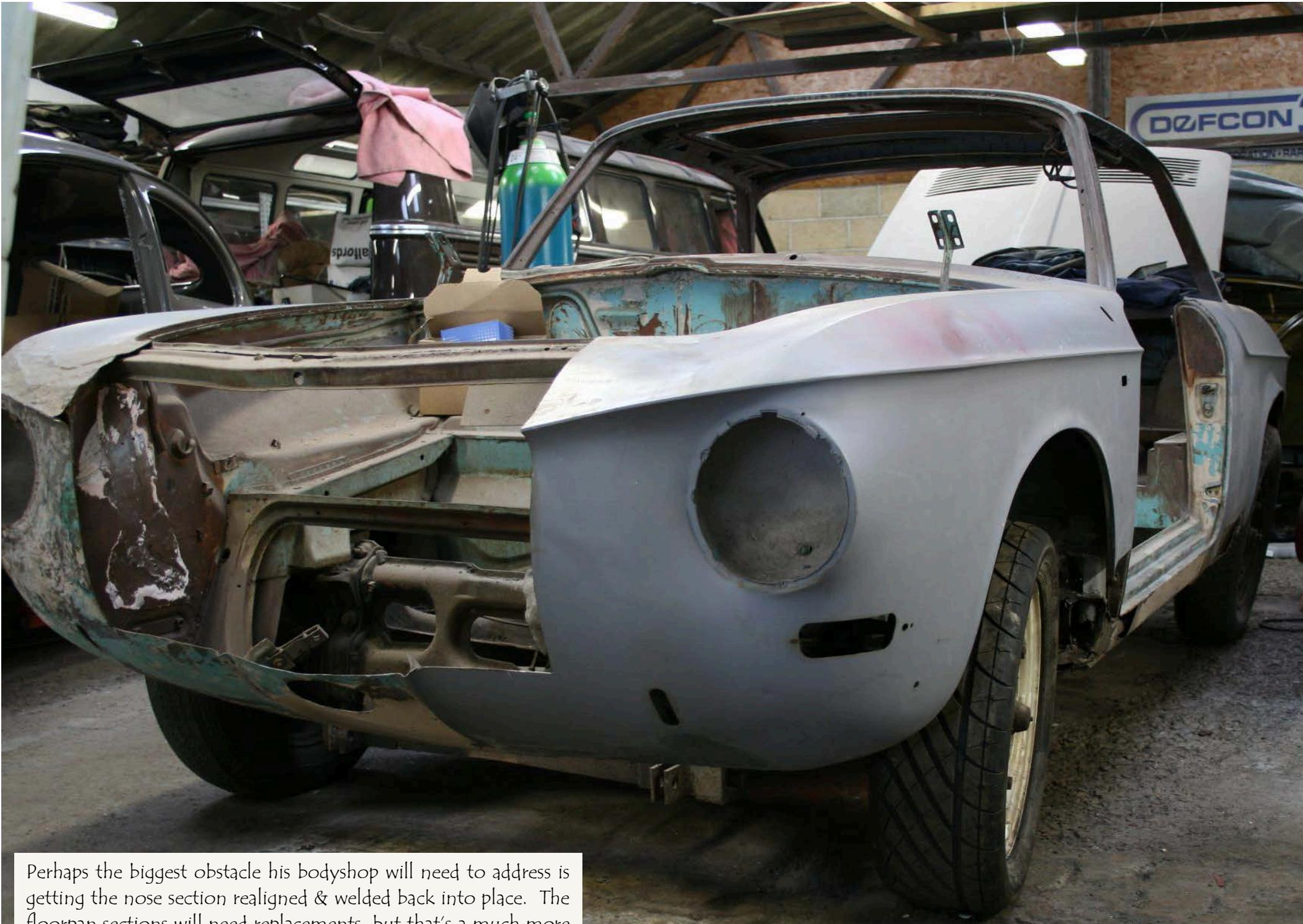
Perhaps the biggest obstacle his bodyshop will need to address is getting the nose section realigned & welded back into place. The floorpan sections will need replacements, but that's a much more straight-forward task which is easily remedied with the Gerson metal T3 floorpans being manufactured in Bogota Columbia.
