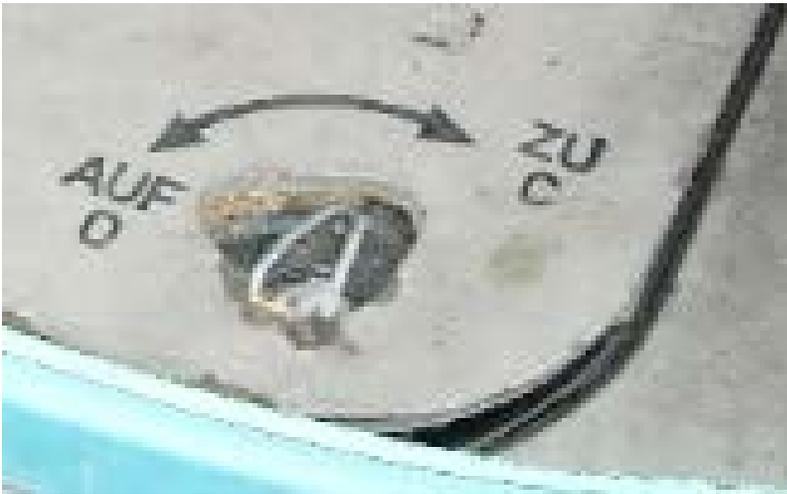
LEFT: Early T34s from 1962-66 featured a trapdoor with O & C (to signify Open & Closed) black lettering printed on the lid to tell owners & repair technicians how to open & close the lid. The trapdoor was not level with the surrounding insulation, perhaps by design to give service technicians a clue as to where the engine was.
