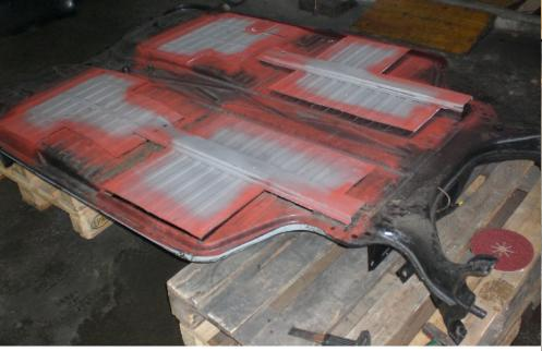
The floorpan sections were sandblasted & the naked chassis was given to body master Paul Goldinger who cut-out the rusty pieces and matched the Belgian floorpan pieces like a puzzle (above). After the welding was done the rust-free chassis was given to Guido's workshop. Guido and Philip spent many hours grinding down the welding seams (below).
