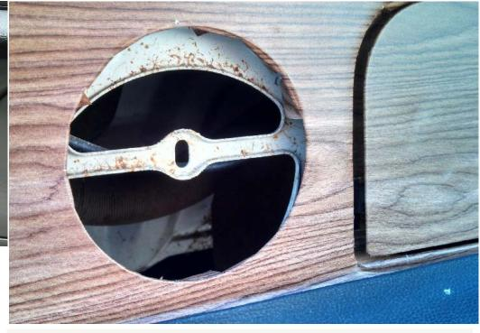
When installing the late style, fitted to T34s from 1967-69, the mounting bracket was already built-in (above), stamped with the new dash design along with the redesigned rectangular radio area. This allowed the speaker cover to be more quickly installed by simply screwing the machine screw into the cover.
