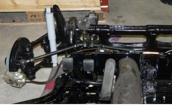
The chassis was painted gloss black in January 2009. Philip worked on cleaning the front & rear axle parts. The front beam was mounted to the chassis (above). The fresh black chassis was looking amazing!
