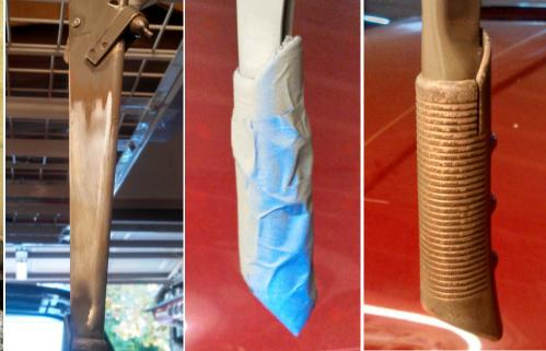
Apply two coats of primer and allow to dry overnight. Then apply two coats of the Anthracite spray paint from Wolfsburg West (Southern California USA) and allow to dry overnight. For a protective shine, spray one coat of clear, as the e-brake handle gets nicked by seat belt buckles & rubbed by forearms when driving.
