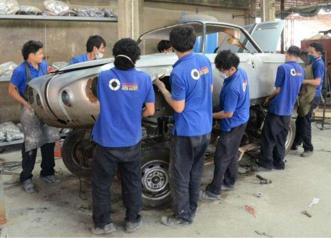
The bodyshop had eleven workers to help lift the body off the chassis. The lower body panels were replaced with fresh metal and the chassis floorpans were also replaced. Once primed it took many hours to get it straight.
