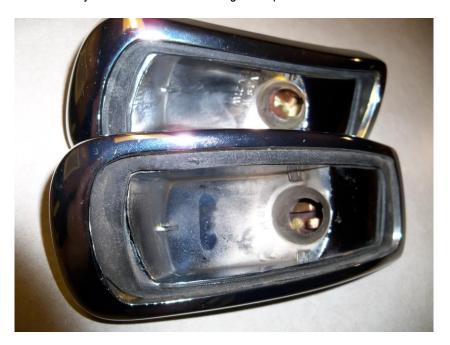
Referring to the picture below, turn signal housings can be easily identified by the 'R' and 'L' next to the leading mounting bolt hole. The housing on the left is a right hand side later European style. The connector cap is white plastic and one of the two terminal mounting connectors is labeled '31', which is electrically **ground** and NOT for use with the grey parking light wire.
