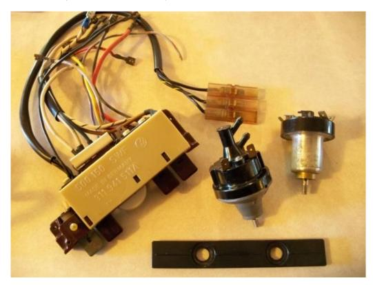
9. Voltage Regulator, 6V version with cabling shown below but the 12V is identical in appearance. The yellow sticker on the side indicates the voltage, so if this identifying label is missing the voltage of the part might be a bit of a mystery and should not be used in your car without being tested first. This part is also used as a replacement part in the Porsche 356, which means that Bosch should keep it available for purchase new.
