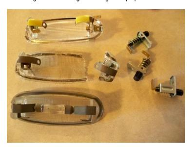
**11.** Left and Right door contact switches, plus the rear decklid contact switch are shown in the picture above, at right. These are only fair reproductions of the original parts and require some rework to fit the car's original mounting holes properly.
