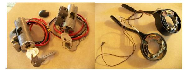
Above right are pictures of turn signal levers. The lever to the lower left is a regular Type 3 unit for use in the North American market. The lever to the upper right is a Type 34 unit and has the secondary ecomomy parking light contacts present for the European market. Notice the thick collar on the Type 34 turn signal lever, which is extremely unique and very rare. The construction
