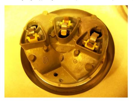
All tail light housings are functionally identical. Though not pictured, a later style tail light housing was produced with a narrow chrome exterior ring and a protruding center stop light reflector. Though not correct, these later lenses can be used on the early tail light housings. Also, the later tail light housings can also be used with the early lenses.
