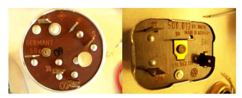
When dealing with used relay that visually pass the test, carefully clean up the terminals on these parts if necessary using very fine grit sandpaper. The idea is to burnish the finish on each relay connector, not burn through it. As water may have already made its way into your relays, it is recommended that you have good spares on hand.
