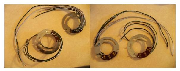
The picture below and to the left is the upper steering column bearing. The bearing housing and steering column is grounded when the horn button is pressed. The wire runs down the inner right hand side of the upper steering column. It is essential that this bearing be in good condition, so replace as necessary. Though pictured with yellow wiring, the insulation color should be brown.
