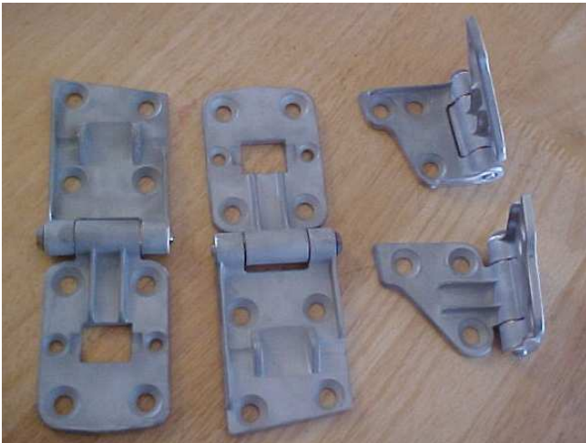
Reworking my hinges even included welding a crack that had developed in near one of the pins.
