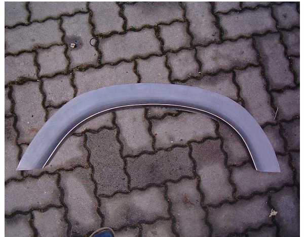
Side view of Lars rear fender arch. Perfect for replacing a rusty or cut wheel arch.
