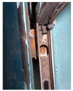
Door Window: Remove the C-clip on the lower window regulator frame (right) and pry the bar over the stud to release it. Remove the six 10mm bolts securing the window regulator to the door frame. Wind the window down
