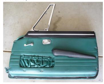
First remove the door hinge screws and drop the doors off from the car. Remove the door check strap block (two screws) and the other hinge screws on the door and bag the parts. Remove the outer rubber seal and door wedge (two screws) at the bottom of the door edge.
