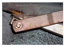
and push the regulator down into the bottom of the door shell. Remove the 10mm lower nut from the vent window frame on the door frame. Side the regulator off the window by pulling it towards the front of the door (below),
