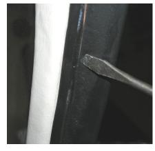
inside edge of the seal into the aluminum channel. Begin at the corner (top of A-pillar) to ensure alignment and then work towards the back of the door window. Trim any excess seal at the bottom of the A & B-pillars with a sharp razor blade for a
