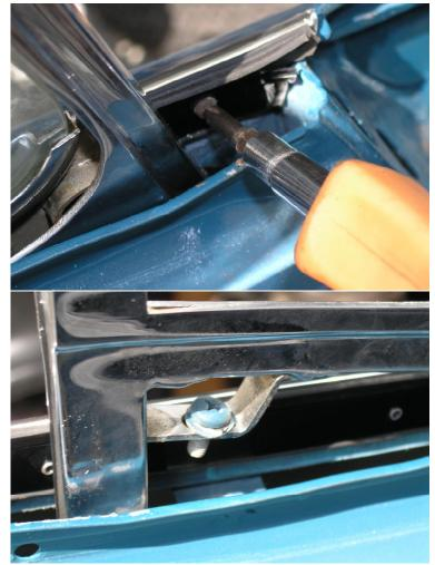
edge. Now install the remaining two window scraper screws to keep it in place. Install the two rubber window guide plugs with the window down & test to make sure they stay in place (right).
