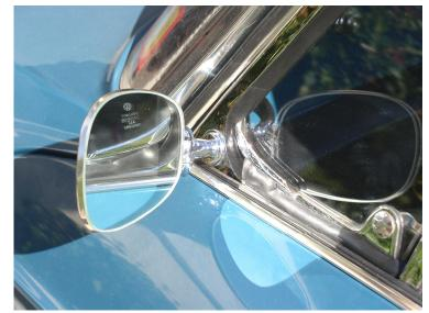
The result is a matching pair of new side mirrors that look 100% original for the 1962-65 T34s. It's not known if the larger mirror head on 1966 T34s can be converted this way as well. And the 1967-69 T34s all use standard Beetle mirrors, so this conversion is also easy.
