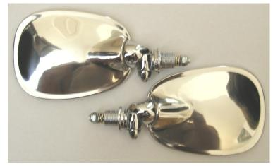
ISP West sells new repro early side mirrors for both left & right sides (above). These mirrors have the T3 mounting stud/threads which cannot be used on a T34. Fortunately the original T34 stud/thread can easily be transferred to the repro T3 mirror. ISP West (<a href="www.vwispwest.com">www.vwispwest.com</a>) #MNVW3-028 (left mirror) & #MNVW03-029 (right mirror) are \$80/pair on eBay or can be ordered directly from ISP West for more.
