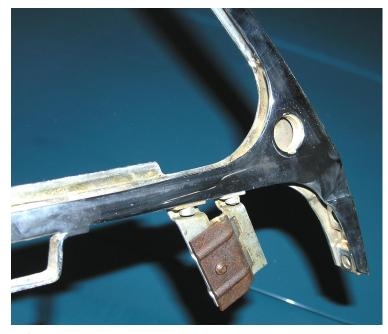
Left-hand-drive owners need to locate a used RHD T34 vent frame (above) from England, Japan, Australia, New Zealand, & South Africa as well as a used T34 mirror (left or right side). Only the stud & thread parts are really necessary for the mirror conversion process.
