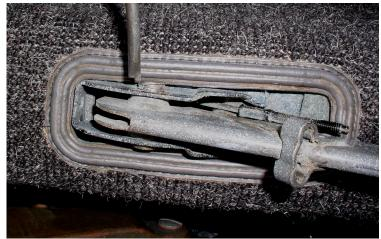
Pry the C-clip off one end of the base stud (above), where the ebrake handle connects to the car. Push the stud out the other side and fit the C-clip again so it doesn't get lost. Now carefully remove the ebrake handle and separate (but attached) tooth'd part.
