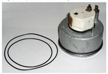
I've found the easiest way to install them is not to remove the gauges but rather to loosen the gauge thumbscrews enough to slip the seals over the gauges. This makes for a quick and easy installation in 5 minutes. They fit snugly around the gauges and when compressed, do not squeeze outside of the trim ring. Perfect, inexpensive, and easy!
