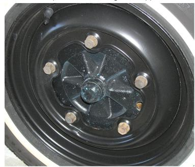
Early model 5-lug T34s (1962-65) have M12x1.5 lug nuts with 20 per car (below). 1966-69 T34s changed to 4-lug and have M14x1.5 lug nuts with 16 per car.
