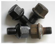
First thing is to remove the lug nuts. The original T34 lug nuts were black but over the years have turned a nasty combination of rust, grease, & grime. Package them up and send them off to a plating shop that specializes in Black-Zinc coatings. The black-
