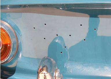
ENLARGING THE SCRIPT HOLES: measure the script tubes and use the same size drill bit to enlarge the holes to fit the tubes. Do one first and test it before finishing the rest.
